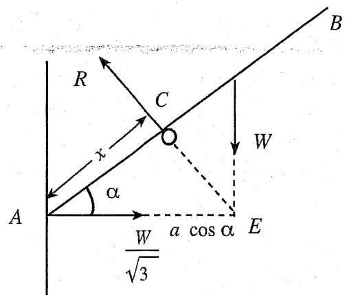
$$\text{C } \frac{W}{\sqrt{3}} \times x \sin \frac{\pi}{6} = W \times (a - x) \cos \frac{\pi}{6} \quad \text{සෙෂ } x = AE \cos \alpha \quad (5)$$
