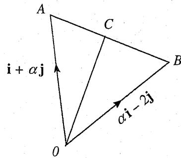
$$\begin{aligned}\overrightarrow{OC} &= \overrightarrow{OA} + \overrightarrow{AC} \\ &= \overrightarrow{OA} + \frac{1}{3} \overrightarrow{AB} \quad (5) \\ &= (i + \alpha j) + \frac{1}{3} [(\alpha - 1)i - (\alpha + 2)j] \quad (5) \\ &= \frac{1}{3} [(\alpha + 2)i + 2(\alpha - 1)j]\end{aligned}$$
