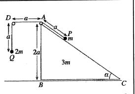
are attached to the two ends of a light inextensible string of length 3a passing over smooth small pulleys fixed at A and D. The system is released from rest with the particle P held on AC and the particle Q hanging freely such that AP = AD = DQ = a, as shown in the figure. Obtain equations sufficient to determine the time taken by the particle Q to reach the floor.
